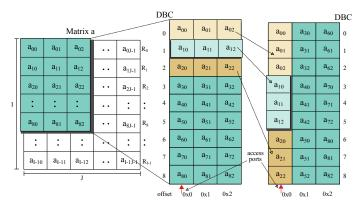
Figure 5. Data layout transformation. Each column in the transformed layout stores 3 rows (clarified with color-coding). In general, each column stores dr rows where dr is determined by the pseudocode in Algorithm 2.
