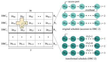
Figure 4. Shifts within a DBC. The figure demonstrates the shifting operation by highlighting one row/DBC (R2/DBC-2) and shows how the access port in the DBC (represented by the arrow) needs to be reset after each iteration of i for the example code in Listing 3. The transformed code in Listing 4 eliminates the overhead shifts by enabling bi-directional accesses.
