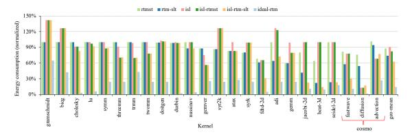
Figure 10. RTM energy consumption in various configurations. All results are normalized to the baseline *identity* configuration. The ideal random access (accesses require no shifts) RTM configuration gives a lower bound on the energy consumption.
