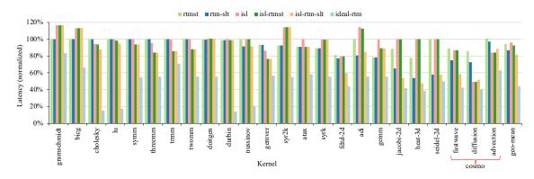
Figure 9. Impact of the schedule and layout transformations on the overall latency/runtime. All results are normalized to the baseline *identity* configuration. The ideal random access (accesses require no shifts) RTM gives a lower bound on the latency.
