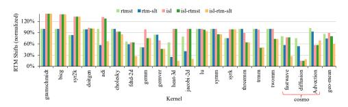
Figure 8. Normalized results of RTM shifts reduction in different configurations. All results are normalized to the baseline *identity* configuration. The figure presents only those kernels where the isl scheduler affects the RTM shifts.
