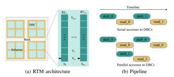
Figure 2. An overview of the RTM architecture. A DBC consists of T (e.g., 32) nanowires and stores K (e.g., 64) T-bit words in a bit-interleaved fashion. The figure on the right shows parallel accesses to DBCs for improved bandwidth utilization and hiding shift latency.
